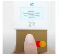
Customers of Crédit Agricole can now use their fingerprint to authenticate contactless payments using a biometric debit card issued by the French bank. Customers have the option of using an enrolment reader at home to register their fingerprint onto their card's chip or they can visit a bank branch to record their fingerprints onto the card.
